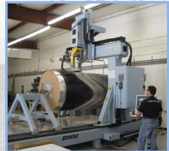
CNC manufacturing of 1200mm diameter, six pole Double-Helix™ rotor coil
