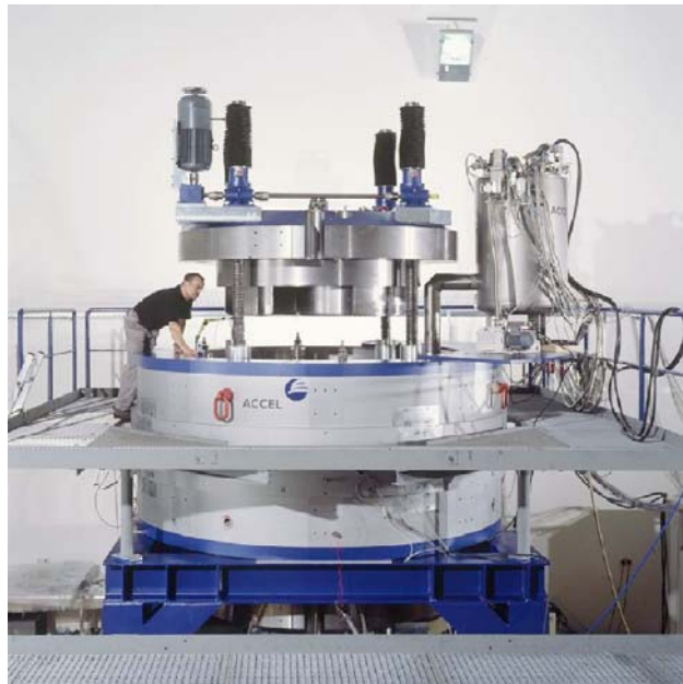
Fig. 19. Picture of the first SC cyclotron for proton therapy (ACCEL Instruments, GmbH, Germany). The upper pole is lifted. On the top right one can see the cryogenic box.
