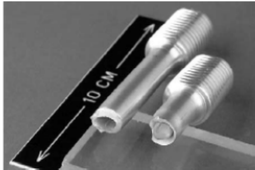
Fig. 8. Fracture of a tensile specimen containing a transverse weld.
