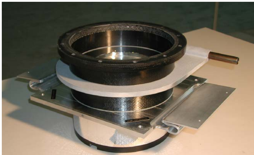
Low heat inleak GFRE support post
