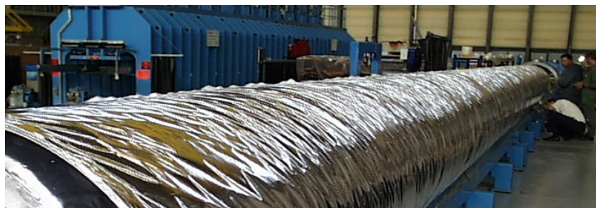
Low heat inleak GFRE support post
