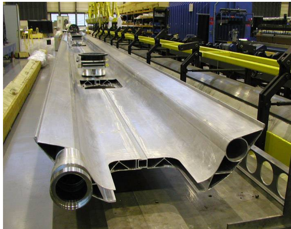
Aluminium extrusion for thermal shield, with built-in cooling channel
