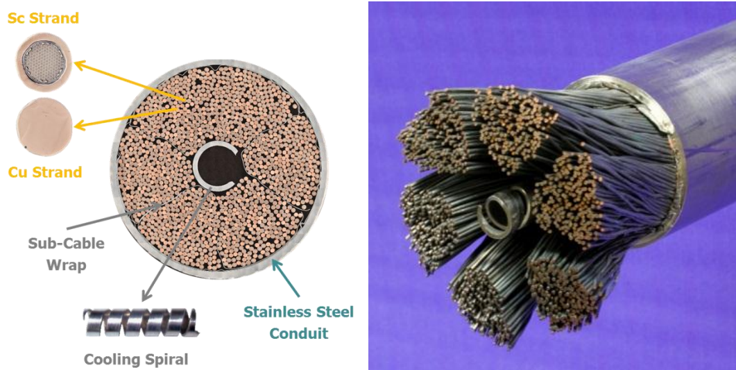
Figure 5. Views of the ITER TF conductors and of its components (courtesy of P. Lee and C. Sanabria, Florida State University).
