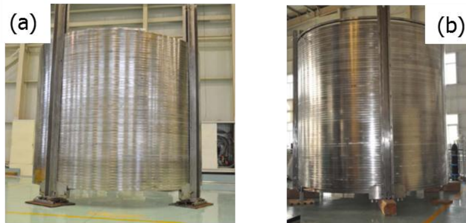
Figure 45: views of first PF conductor ULs manufactured in China: (a) 740 m long Cu dummy UL and (b) 910 m long Cu dummy UL (Courtesy of Y. Wu, ASIPP).
