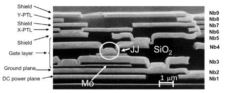
**Fig. 1.** Cross section of the advanced fabrication process as described in [2]. Beside the four layers from the standard process (Nb2 - bottom ground plane, Nb3 - base electrode, Nb4 - counter electrode, Nb5 – top ground plane), the layer package includes additional layers for dc power supply and for strip-line interconnects in both x- and y-direction (photo - courtesy of M. Hidaka).
