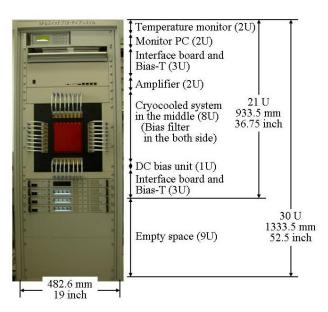
Fig. 2. The cryocooled network switch installed in a 19 inch rack (photo – courtesy of Y. Kameda).
