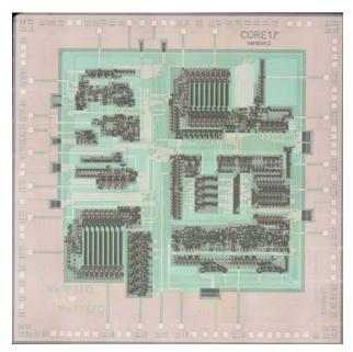
Fig. 3. Photograph of the 8 bit serial microprocessor Core1 $\gamma$  (photo - courtesy of A. Fujimaki).
