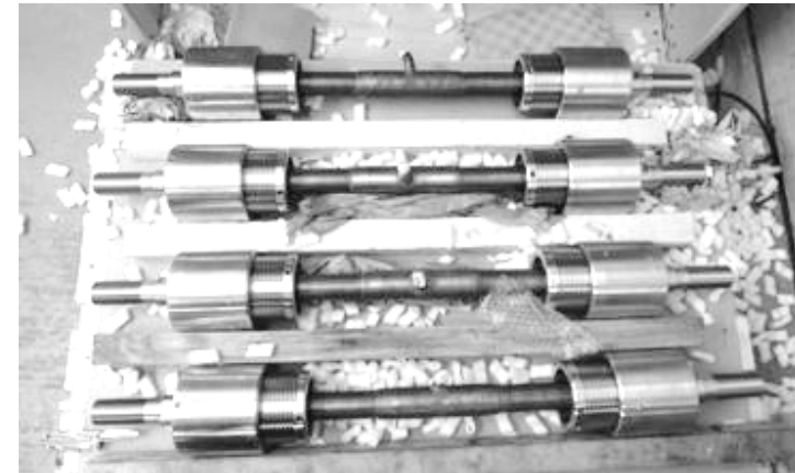
Fig1. TF inlets fatigue test samples
