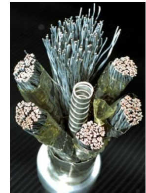
Fig. 5 Cable in conduit made of 900 Nb 3 Sn strands in multistages with central channel into 316LN jacket
