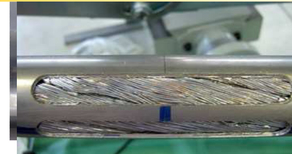
Fig 2. Fabrication of Helium inlet onto conductor
