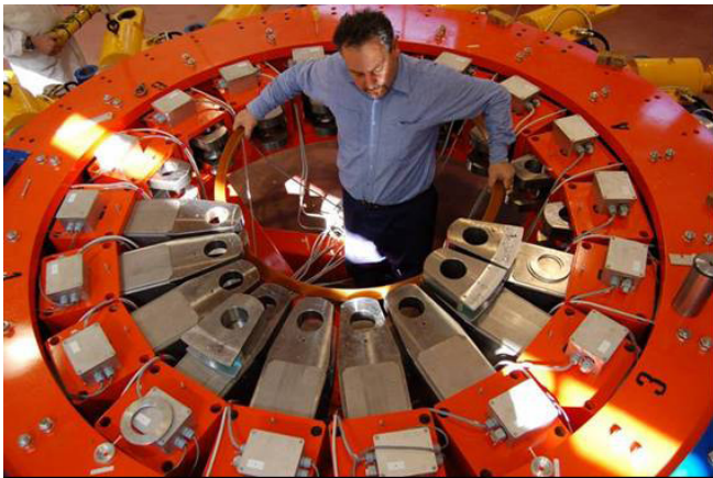
b) Testing jig installed at ENEA (It, Frascati) for mock-up rupture test
