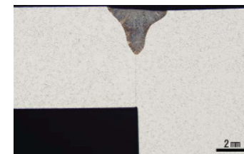
b) Typical closure cover laser welding bead
