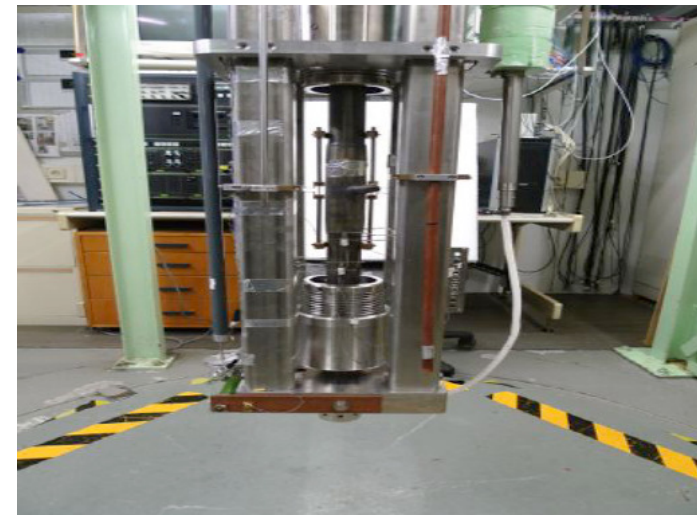
Fig 2. Fatigue tensile test machine layout ( courtesy of KIT)
