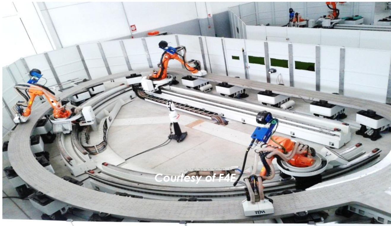
Fig.1 Laser welding of the cover plates with 3 welding robots
