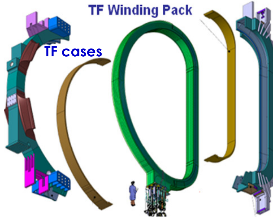
Fig.3 Winding pack formed of 7 radial plates containing conductors.
