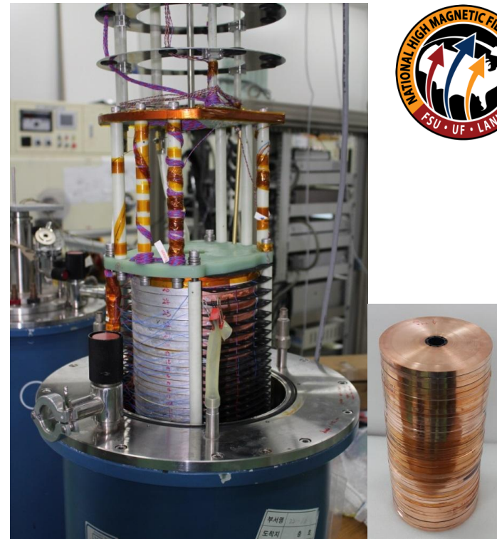
26 Double Pancake Coils Stacking
