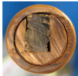
Tapes dislocated with twisting.
