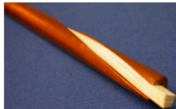
Tapes dislocated with twisting.
