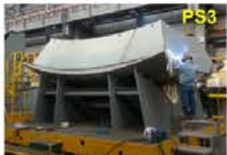
PS3 ◀ Start welding after inner and outer jigs for inner shell of equatorial segment (PS3)
