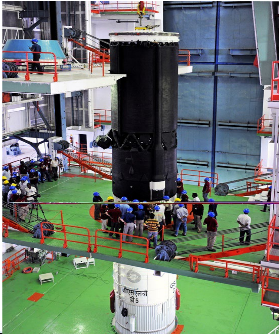
Three Stage ( Solid, Liquid & Cryogenic) Launch Vehicle with Cryo Engine
