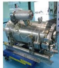
Field flatness 92% dressed cavity with tuner and coupler in HTS
