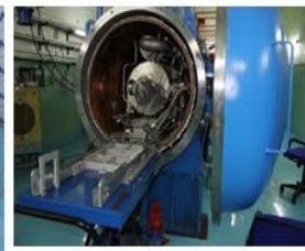
Field flatness 92% dressed cavity with tuner and coupler in HTS
