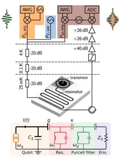
Conventional method for superconducting qubits requires pulsed microwave tones generated at room temperatures
