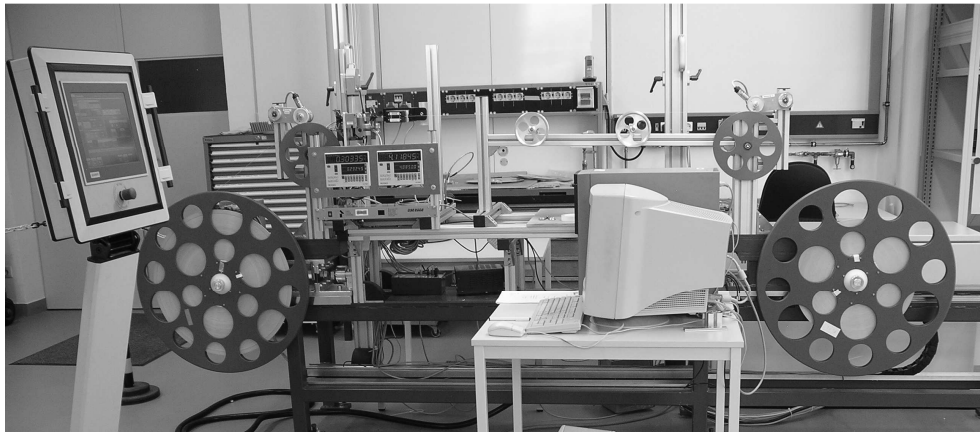
Figure 5. Conductor test set-up to check HTS width, thickness, and insulation
