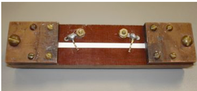
Figure 1. Sample holder used in pulsed current experiments. All samples measured were 10 cm long, with the first 2 cm at each end overlapping with current contacts (thick copper blocks). Indium foil was used to ensure low contact resistance between copper and sample. Voltage contacts separation was 4.2 cm.
