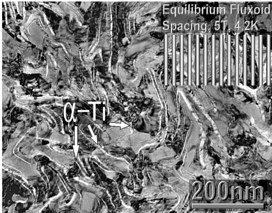
\alpha -Ti ribbons in a Nb-Ti alloy (Larbalestier & Lee)
