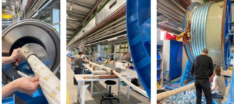
Fig.8. MgB_2 Feeder cable for accelerator (By courtesy of Prof.A.Yamamoto(KEK))
