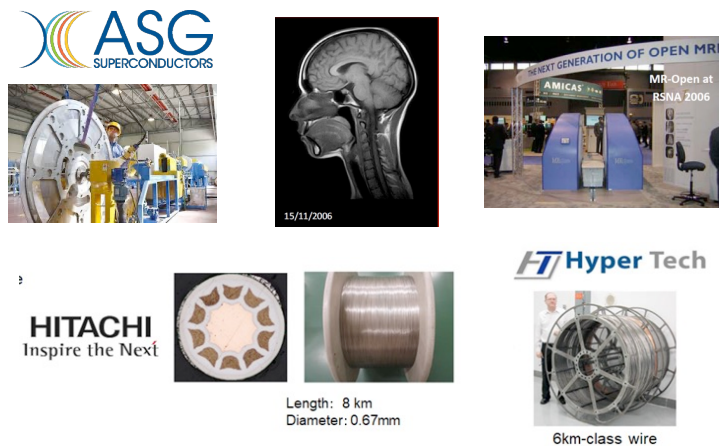
Fig.7. MgB_2 wires and MRI application
