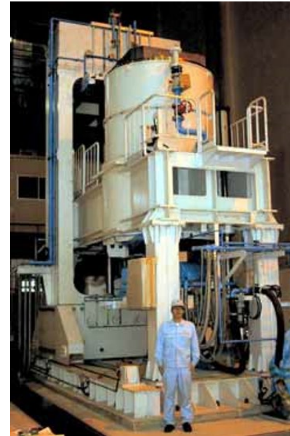
Sumitomo Electric OP furnace for Bi-2223 - 200 bar cold wall – in use for 15 years
