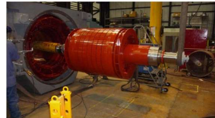
Figure 7. 3.6 MW 1800 RPM ship propulsion motor. © 2015 IEEE. Reprinted, with permission, from [22].
