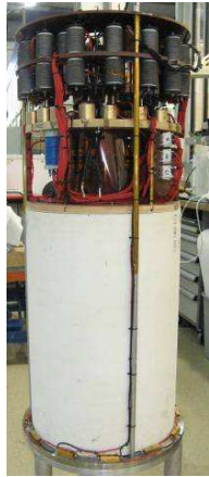
Fig. 2. Photo of the Oxford Instruments 20 T / 78 mm bore LTS magnet outside its cryostat.
