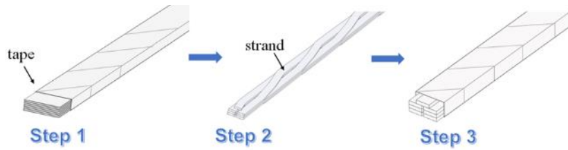
Schematic illustration of the transposed cable and the fabrication steps
