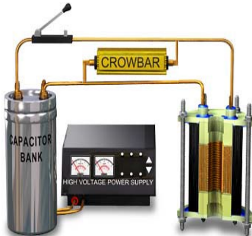
Capacitor-bank driven pulsed magnets
