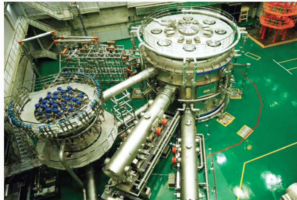
KSTAR –South Korea, 2008, All superconducting TF and PF coils (30 in total, 26 coils are made of Nb 3 Sn and 4 of NbTi).
