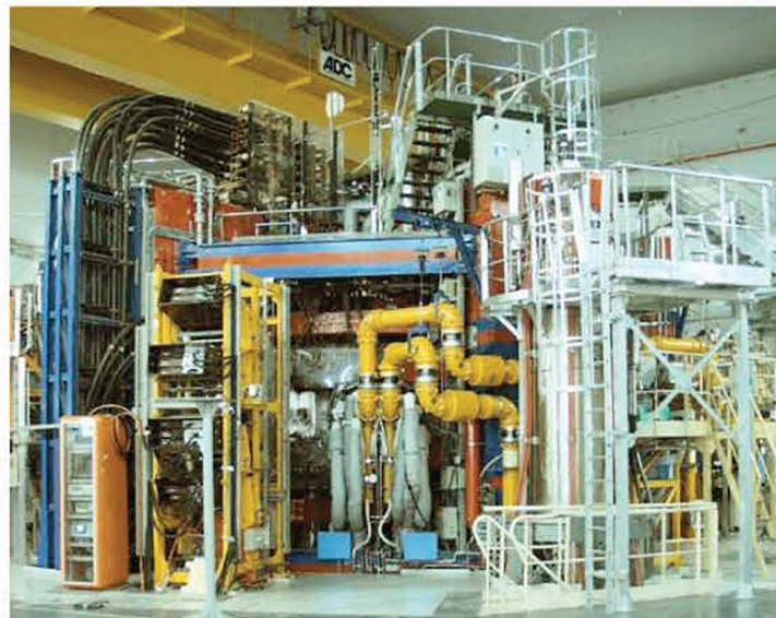
TRIAM-1M Kyushu University 1986 Nb 3 Sn superconductor in its 16 D-shaped TF coils, cooled by pool boiling liquid helium
