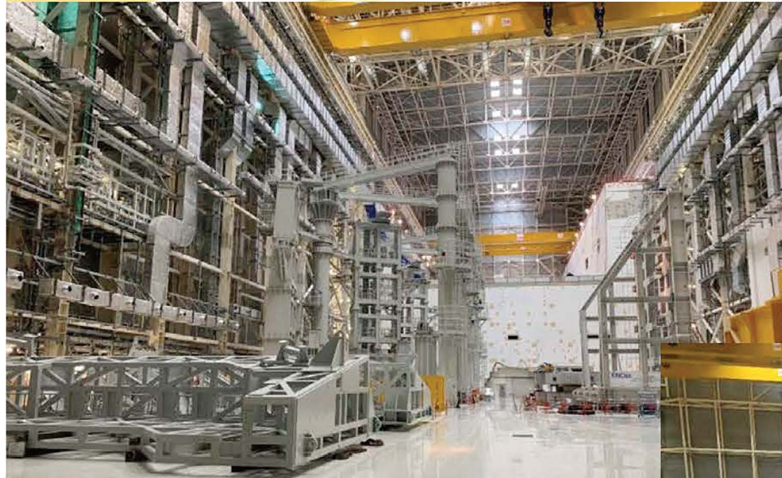
Main assembly hall June 2020 Sub Sector Assembly Tools (SSAT) Each for mounting 2 TF coils and 1 VV sector
