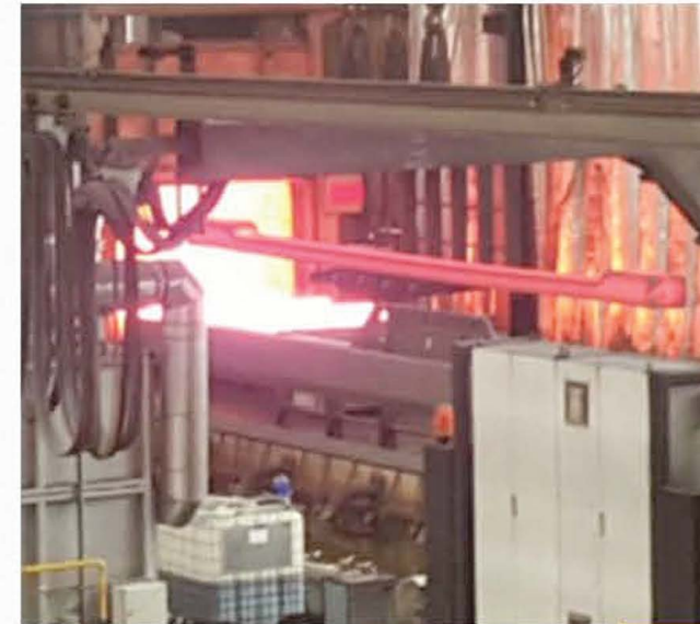
2015-16 Offset forging of a 12m CS tie plate
