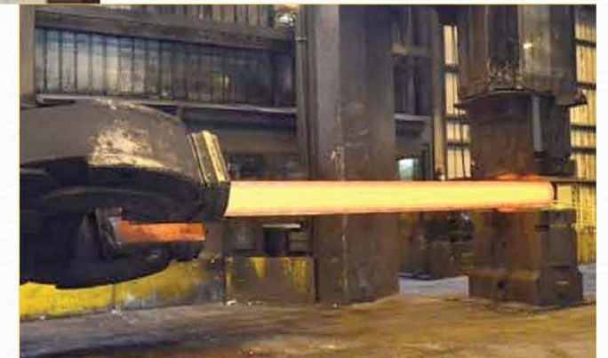
2015-16 Offset forging of a 12m CS tie plate
