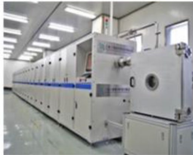
Coating and growth of the Superconducting layer
