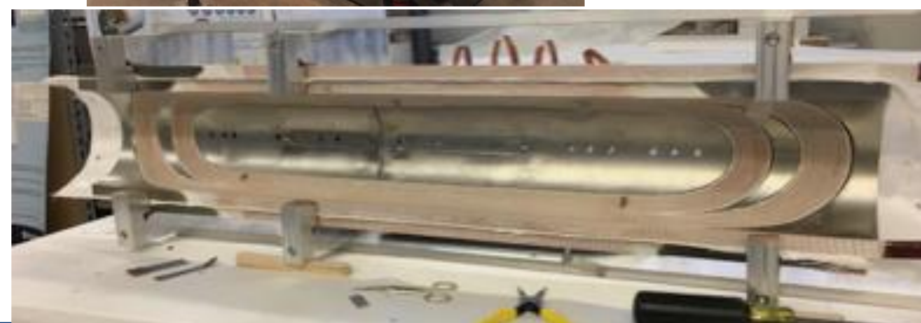
60-mm aperture, 4-layer graded coil
