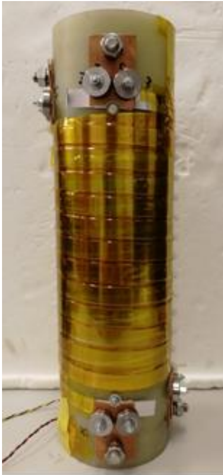
Helical bifilar SFCL coil
