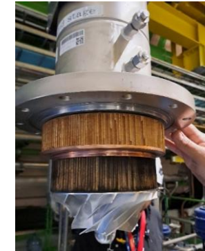
Replacing a cold compressor impeller in LHC
