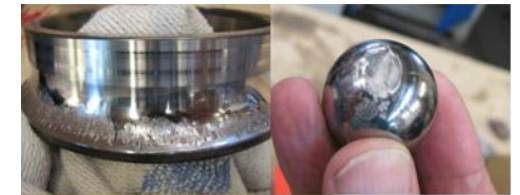
Damaged ball bearing
