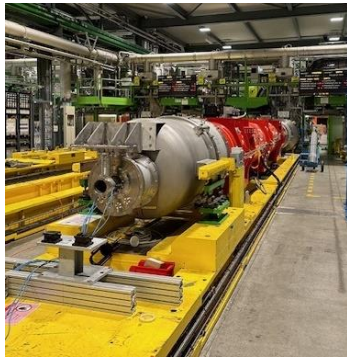
Horizontal magnet tests in SM18
