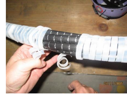
NbTi cable of LHC SC link
