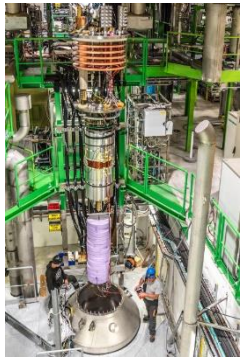
Vertical magnet tests in SM18
