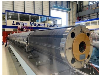
Nb 3 Sn magnet for HL-LHC (1.9 K)
