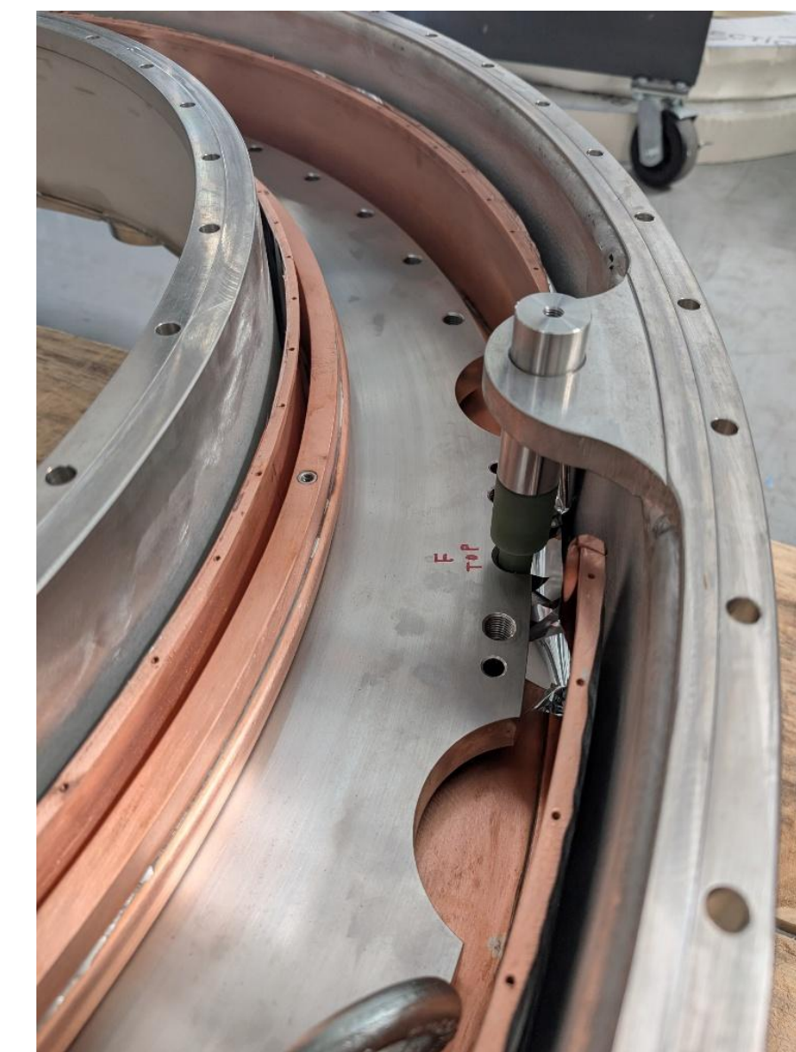
Fitting of magnet former within cryostat and thermal screens
