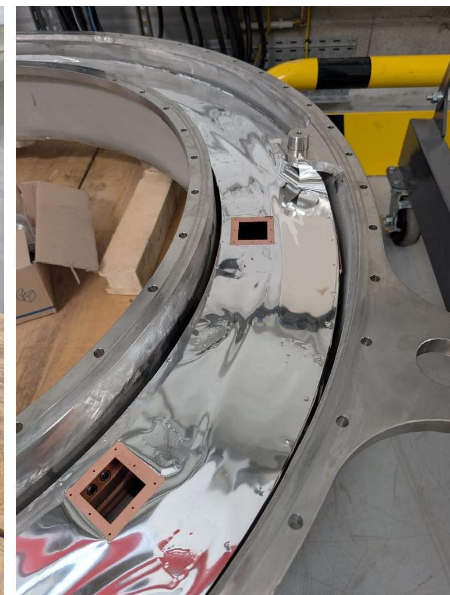
Fitting of magnet former within cryostat and thermal screens
