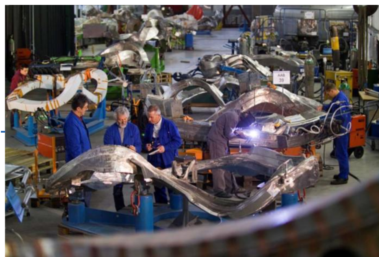
Welding of the coil case
