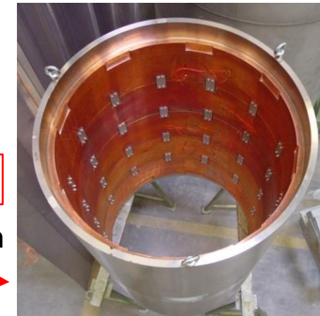
25.5 T Polyhelix coil, \varnothing_{\text{ext.}} = 372 \text{ mm}
