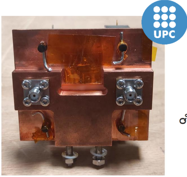
Parallel Plate Resonator at 1 GHz \text{Al}_2\text{O}_3 dielectric sandwiched with 2 delaminated REBCO samples
