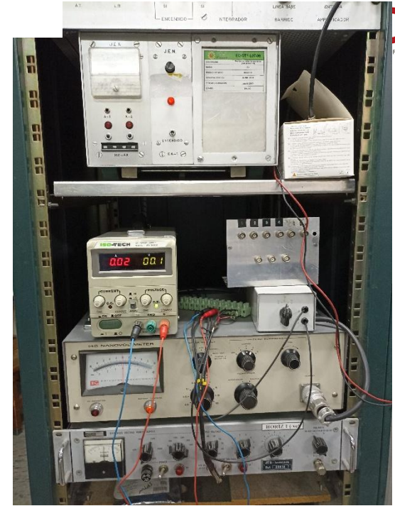
In-situ sample resistance monitoring during irradiation at RT
