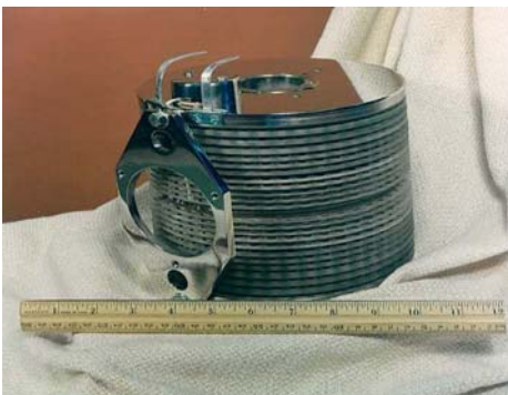
Fig. 16. 11 T split magnet for horizontal or vertical mounting.
