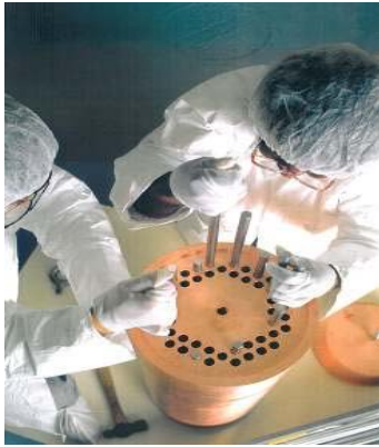
Fig. 8. NbTi rod assembly into copper billet at IGC.
