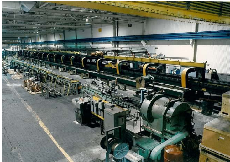
Fig. 24. The 120-m-long draw bench acquired for large-volume NbTi wire manufacture.
