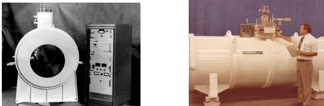
Fig. 23. Large-bore 2 T NbTi magnet with its electronic control panel (left); IGC's precursor to NMR large-bore magnet (right).
