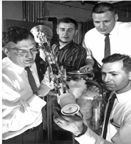
Fig. 2. 101 kGauss, Nb 3 Sn magnet, fabricated and tested by: L. Martin, C. Bruch, M. Benz and C. Rosner (left to right)
