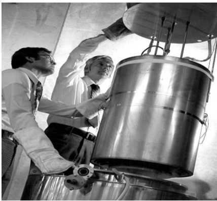
Fig. 20. Test of 3,000 HP S.C. motor for ship propulsion
