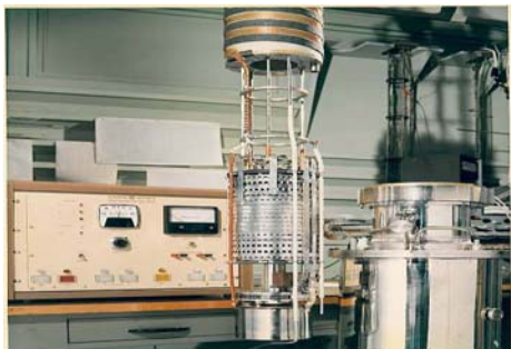
Fig. 10. Early 10 T tape magnet powered with “Buchhold” Flux Pump.
