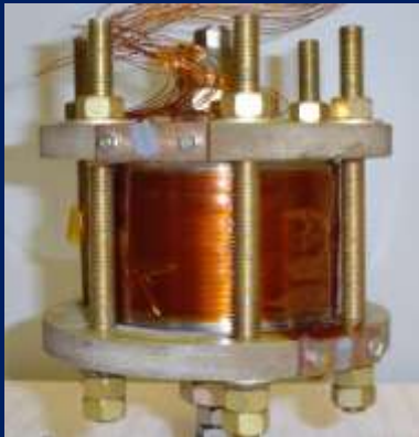
0.0001 m 3 HF insert model ~ 200 A
