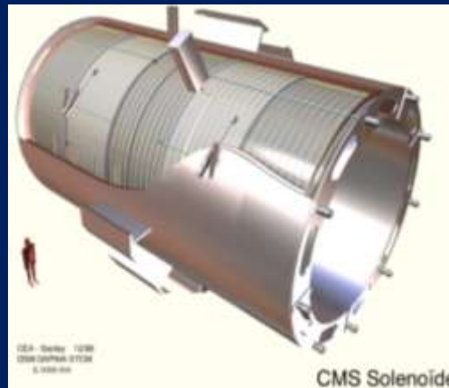
400 m 3 HEF detector magnet 20 kA @ 4 T, 2.6 GJ
