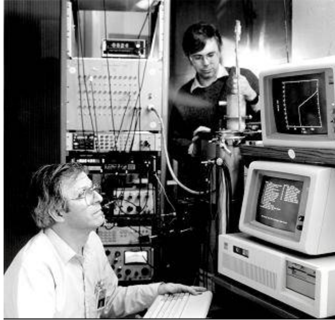
Fig. 6. Bob Laibowitz and the late Roger Koch shown in 1987 taking resistive transition data for an epitaxial YBaCuO superconducting film.
