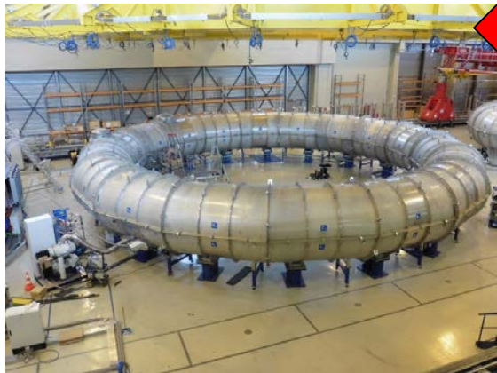
Double pancake winding and insulation
