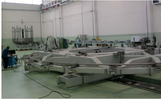
Winding of double pancake according to nominal trajectory
