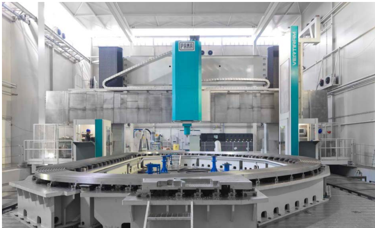
Final machining with portal machine on nominal trajectory at 20 \pm 1 \text{C} (at CNIM)
