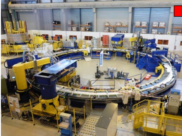
Double pancake winding and insulation
