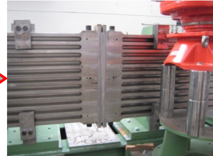
Forged segments are butt-welded (NG GTAW or LV EB) into larger sectors at SIMIC
