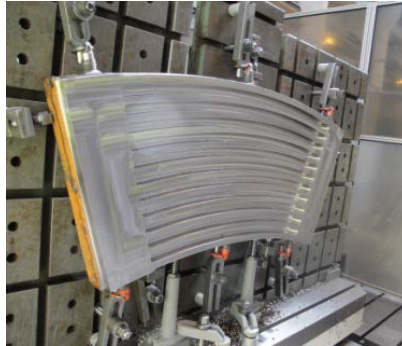
Forged segments are pre-machined (5mm over metal) at CNIM
