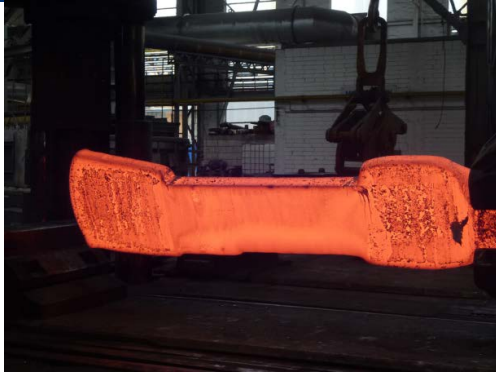
6 segments of ITER grade 316LN are forged for each RP (Courtesy by Thyssen)
