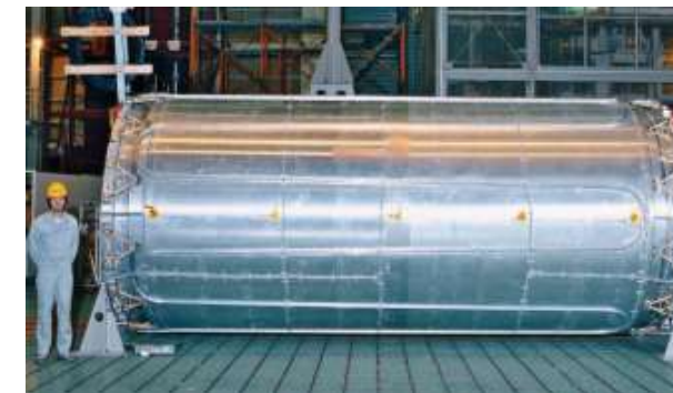
25 m 3 ATLAS Solenoid 8 kA @ 2 T, 40 MJ
