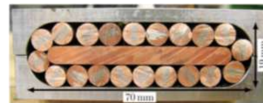
Swiss Plasma Center: Twisted Stacked Rectangular CICC
