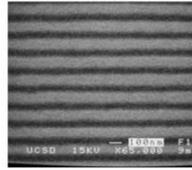
SEM Photo of the mask structure used for implanting a 100-junction array
