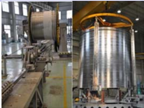
Winding of PF2/3/4 conductor
