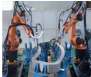
Automatic welding of coil case
