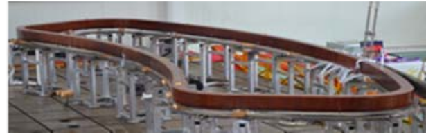
Dummy coil after VPI
