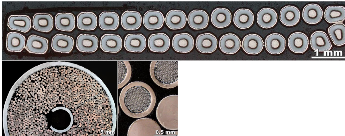
Nb-Ti strand and monolith cross-sections just from one manufacturer: Bruker EST (Courtesy Manfred Thoener)
