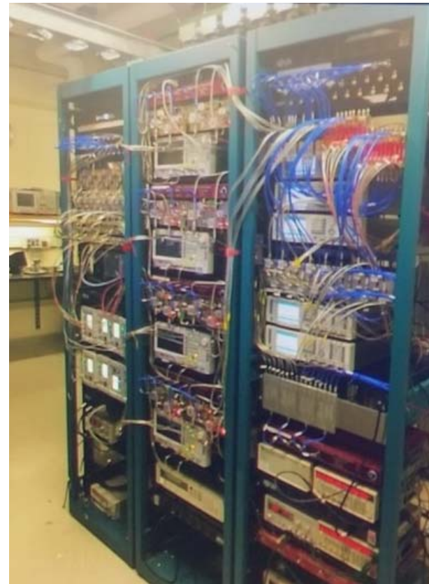
IBM 20-qubit system setup (J. Chow, Q2B conf., Dec. 2017)
