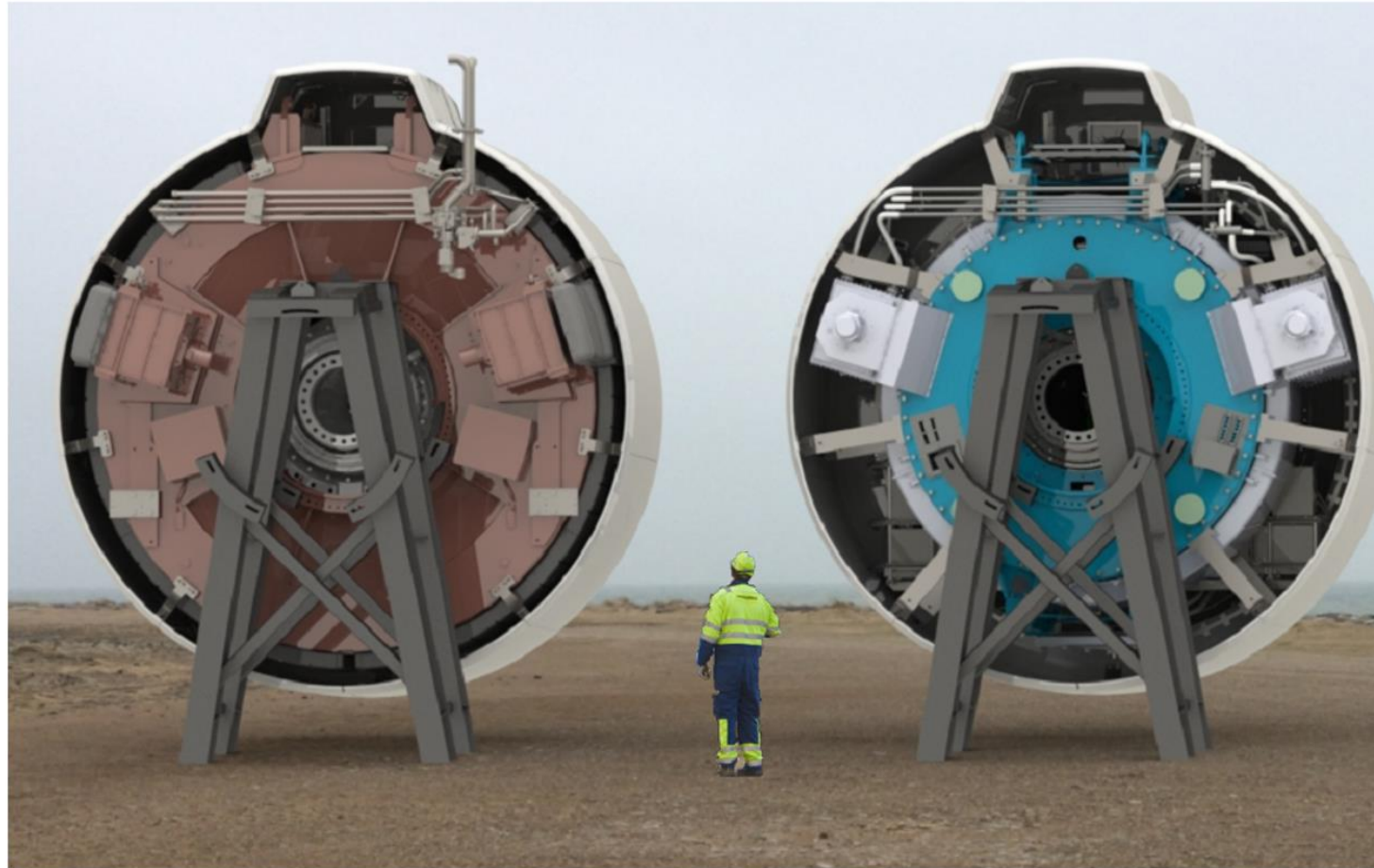
Fig. 1: EcoSwing generator (right) next to the original permanent magnet generator (left) in a CAD generated image. Note the considerably smaller diameter of the EcoSwing.
