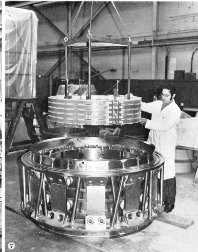
FIGURE 7. Superconducting d.c. generator field coils being fitted into coil support structure.
