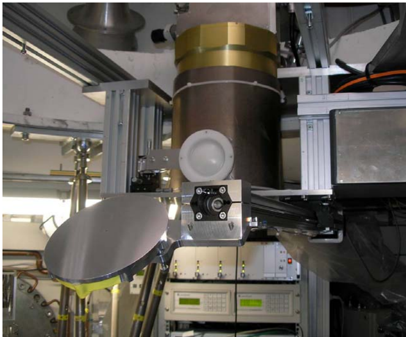
Fig. 5. The SABOCA cryostat is mounted at APEX telescope cabin.
