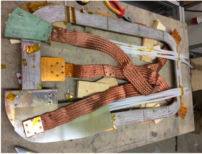
Fig. 4. Setup of the SC4, including copper braids
