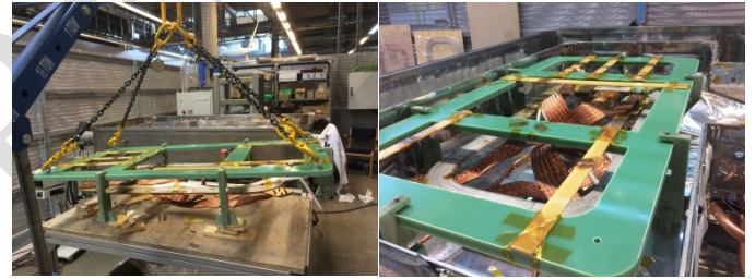
Fig. 6. SC4 set up prior test. Left: lifting process of the SC4 and the frame. Right: SC4 in the cryostat before to be tested.
