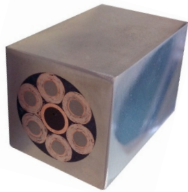
Demonstration conductor: 6-around-1 Conductor-in-Round-Core (CORC) Cable-in-Conduit Conductor (CICC)
