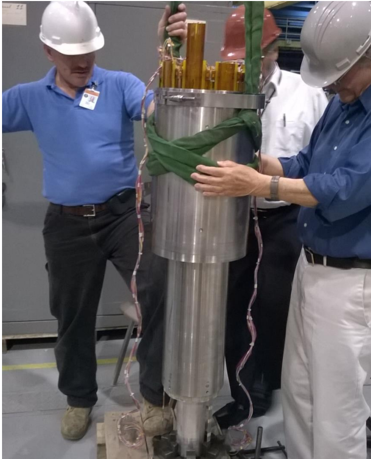
Outer inserted over inner coil
