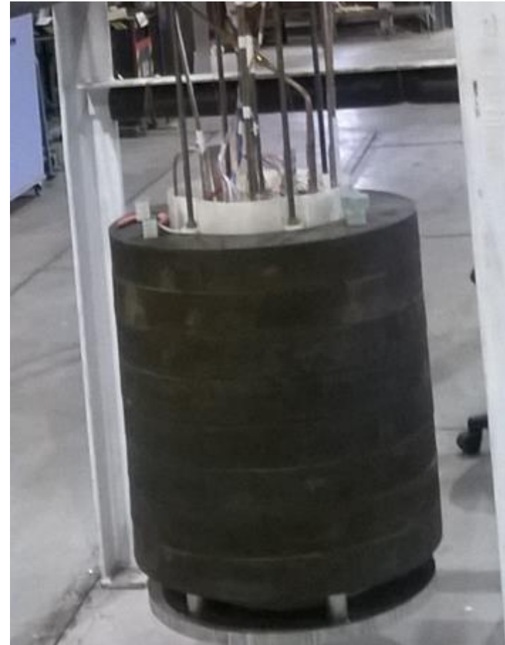
SMES coil in iron laminations
