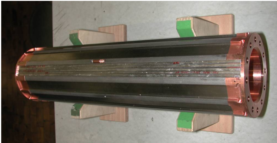
Fig. 2. HTS part mock up of the W7-X HTS current lead developed at the Forschungszentrum Karlsruhe.
