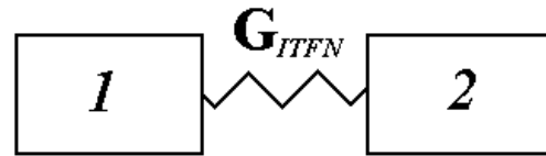
Fig. 2. The simplest model for internal thermal fluctuations assumes two systems, 1 & 2 connected by a thermal conductance G_{ITFN} .
