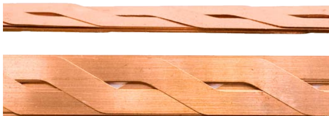
Fig 1. Close up photographs of YBCO Roebel cable.
