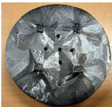
Fig.3 Bulk Y-Ba-Cu-O sample melt-processed with the maximum temperature of 1058°C using MgO-doped Nd123 seed crystals. One can see that four domains were fully grown in the entire bulk.
