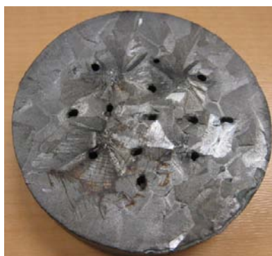
Fig.1 Bulk Y-Ba-Cu-O sample melt-processed at the maximum temperature of 1050°C using Nd123 seeds, exhibiting polycrystalline structure.
