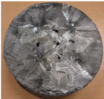
Fig.2 Bulk Y-Ba-Cu-O sample melt-processed at the maximum temperature of 1055°C using Nd123 seeds. Grains grew larger but the Nd123 seeds were dissolved.
