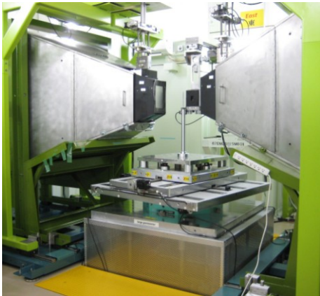
Figure 6: Neutron diffraction measurement facility at the BL-19 (TAKUMI) of J-PARC MLF.
