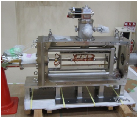
Figure 8: Cryogenic load frame up to 50 kN from 6 K to 300 K.
