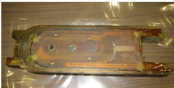
Figure 5: Picture of a dummy sub-scale coil impregnated with the new cyanate ester base resin.
