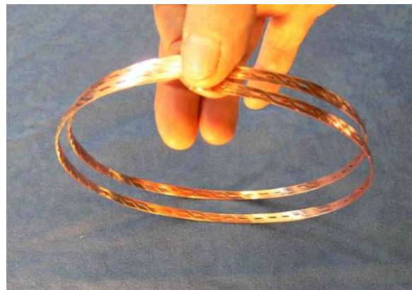
Fig. 4. A finished length of YBCO Roebel cable
