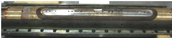
Figure 5: \text{Nb}_3\text{Sn} dipole coils impregnated with ceramic binder after winding and curing (top) and a quadrupole coil cured with ceramic binder after reaction (bottom).
